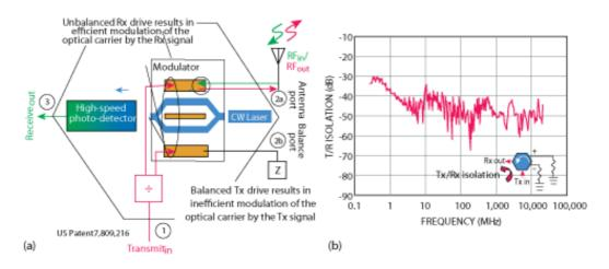
Mismatch is managed by connecting a variable impedance to an additional 'antenna balance' port which replicates antenna impedance versus frequency.
