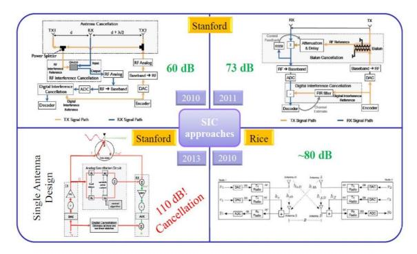
Research at Stanford University was also referenced showing the improvement made over the past three years with a claimed 110 dB now being available coupled through a single antenna.
