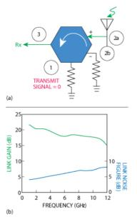
At frequencies where the impedance at the two bidirectional ports are equal, the transmit signal at Port 1 is routed to the antenna connected to port 2 and the signal received by the antenna is routed to Port 3. Port 3 is isolated from Port 1 because the portion of the transmit signal that is reflected by the antenna back into Port 2 (a) is balanced by the transmit signal reflected back into the 'balance' port 2(b) by the impedance connected to the fourth port.
