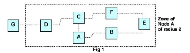
The box defines a zone in which the minimum distance from any device to any other device is never more than 2 hops. Nodes B through F are within the routing zone of A, node G is outside A's routing zone.
